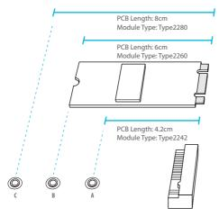
3. Move the stando based on the module type and length. The standoffs is placed at the nut location D by default. Skip Step 3 and 4 and go straight to Step 5 if you are going to use the default nut. Otherwise, release the stando by hand.
