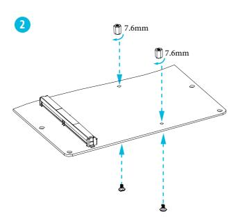
\*Before installing a Type B+ MXM card, please replace the 5mm standoffs with the 7.6mm standoffs.
