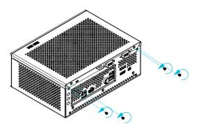
2. Slide the top cover outward and then lift it off the chassis.
